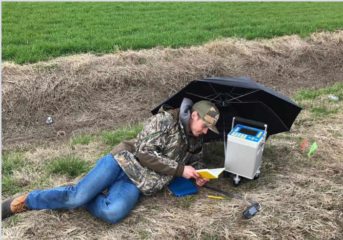
Brooks Rosandich collecting gravity data to detect faults on Charleston Uplift, Mo. Brooks is an MS student in Geological Sciences, working with Professor Edward Woolery.
