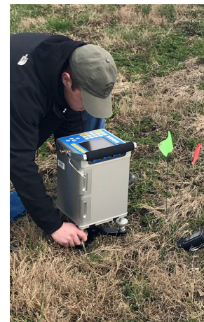
Drew Burford uses gravity data to detect faults on Charleston Uplift, New Madrid Seismic Zone.
