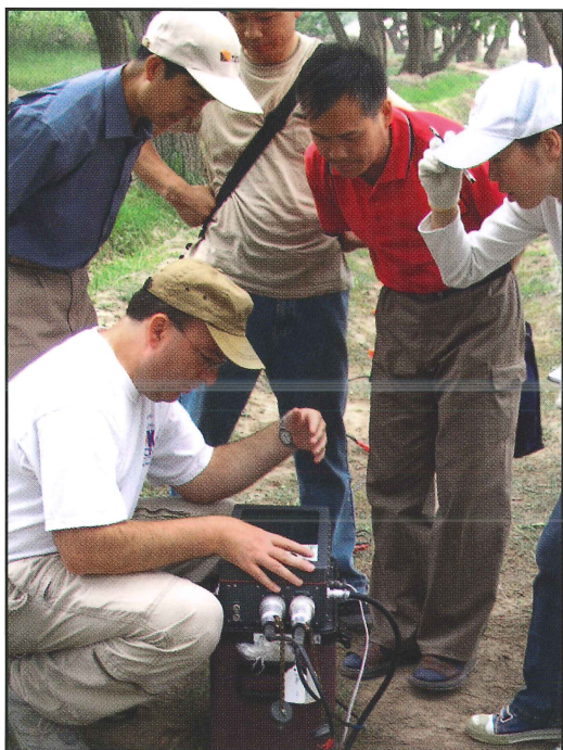
UK researchers successfully demonstrated high-resolution seismic S-wave reflection techniques to their Chinese colleagues during field investigations in Gansu Province this past summer.
